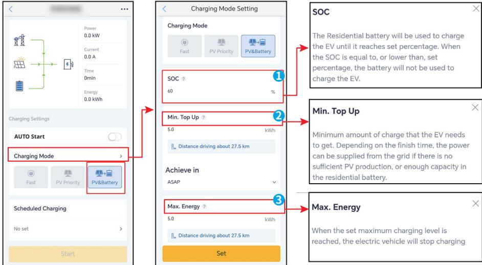
The image shows a three-step process of navigating through the vehicle's charging settings. On the left, the main 'Charging Settings' screen is shown with 'Charging Mode' selected. In the middle, the 'Charging Mode Setting' screen is shown with three settings highlighted and numbered: 'SOC' (1), 'Min. Top Up' (2), and 'Max. Energy' (3). On the right, three callout boxes provide detailed explanations for each setting.
